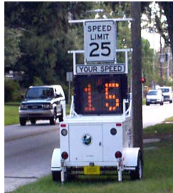
Speed display trailer in action on a residential street
